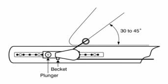
Position the slide on the track ensuring the plunger end of the slide is aft and the becket on the slide is facing down. (This may need to be adjusted depending on whether it is fitted on port or starboard side of the boom. The eye will rotate but may require the use of pliers to carry out this operation)
