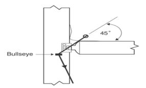
Use the bullseye as a template to mark the position of the two fixings with centre punch then, remove bullseye and drill using a 3.3mm drill before tapping using the 4mm tap. . After securing, the screws can be removed and the surplus length inside the boom cut off, to prevent possible snagging of internal control lines on the sharp ends of the screws.
