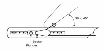
Lower the main halyard to the correct position for reefing and reef mainsail. If correct, mark the halyard at the position of the cleat with permanent marker.
