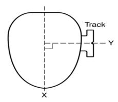
Remove track, drill using 4.2mm drill and tap using 5mm tap then secure in position using 5mm machine screw
