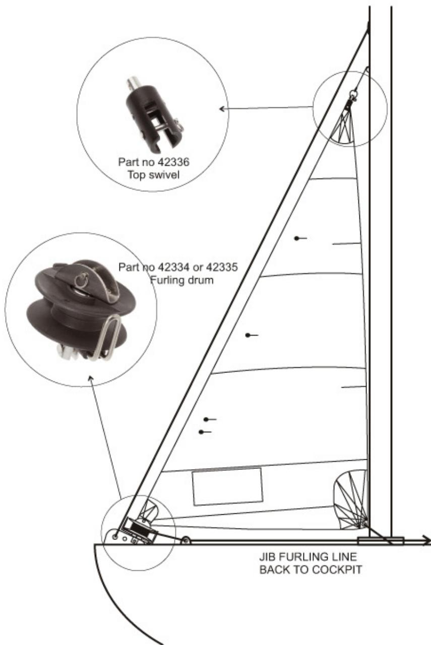
The jib requires a fixed wire luff and two attachment points at the bow, one for the forestay and one for the furling drum, separated enough that they do not touch. Attach
