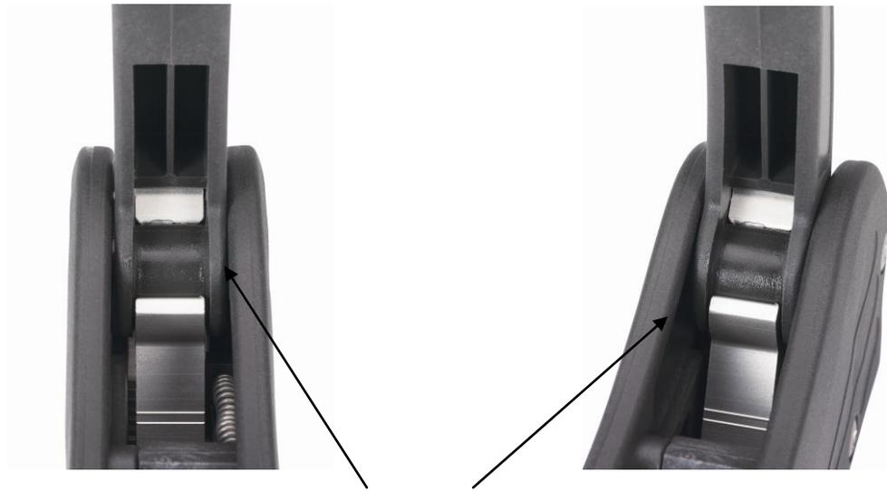
*Rope Clutches - Grease handle and pivot with silicone grease in the Springtime*
