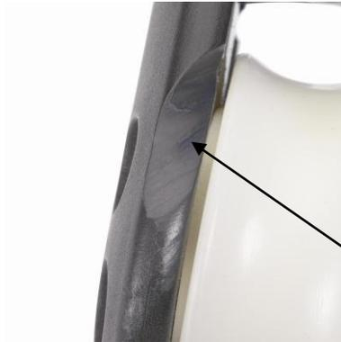
*Block with excessive side plate wear*
