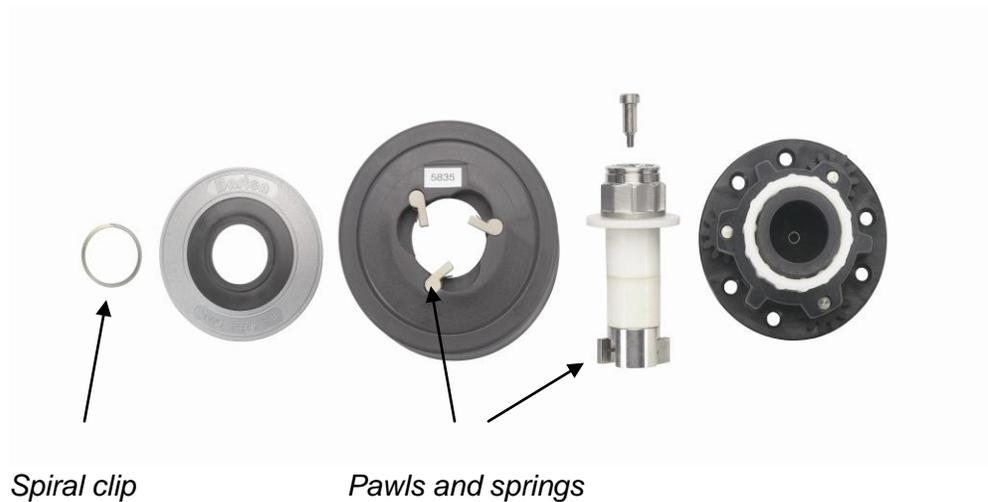
*Winches - Breakdown of the two speed winch components showing spiral clip and drum with pawls and springs*
