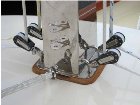
Plain bearing blocks fitted at the mast base
