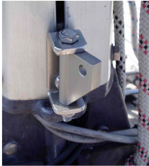
Photo 2 (right): A lug slides inside the sail track and allows the mast bracket be fitted without drilling the mast.
