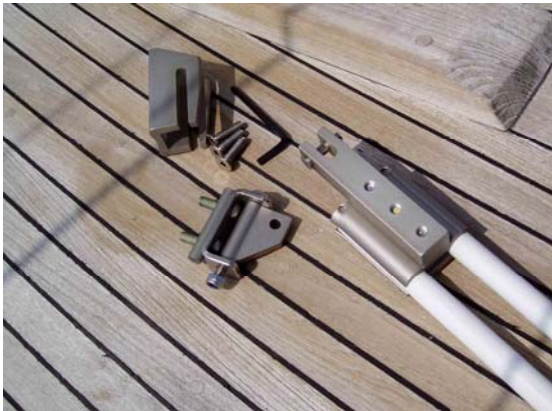
Photo. 1 (above): The boom fitting (top), mast bracket (center) and a clamp at the end of the fiberglass rods.
