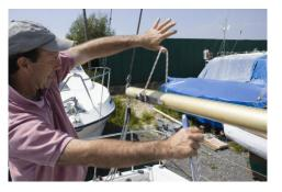
Position the slide on the track ensuring the plunger end of the slide is aft and the becket on the slide is facing down. (This may need to be adjusted depending on whether it is fitted on port or starboard side of the boom. The eye will rotate but may require the use of pliers to carry out this operation)
