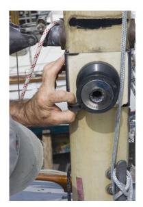
Use the bullseye as a template to mark the position of the two fixings with centre punch then, remove bullseye and drill using a 3.3mm drill before tapping using the 4mm tap. . After securing, the screws can be removed and the surplus length inside the boom cut off, to prevent possible snagging of internal control lines on the sharp ends of the screws.
