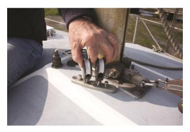
Attach the correct sized double tang blocks (Size 3 on the Centaur part# 03 090) to the swivel posts using the plastic spacer washers provided for a snug fit then lead your control lines through.
